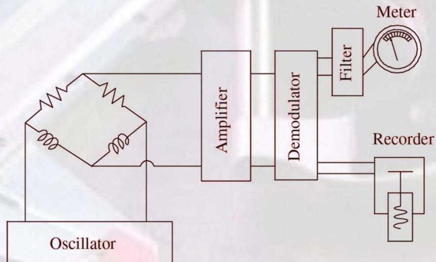
**Fig. 9.11** Bridge circuit and electronics
