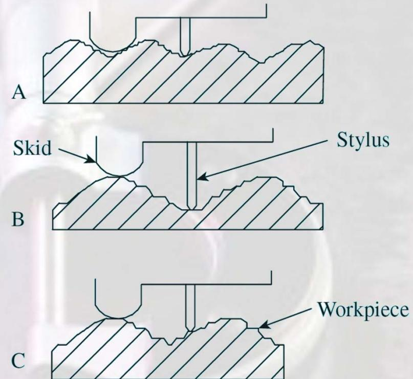
Fig. 9.12 Phase relationship between the skid and stylus
