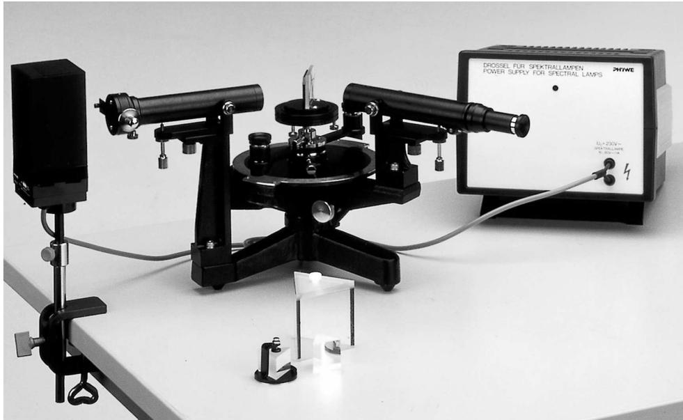
Figure 7: Experimental set-up for determining dispersion in prism.
