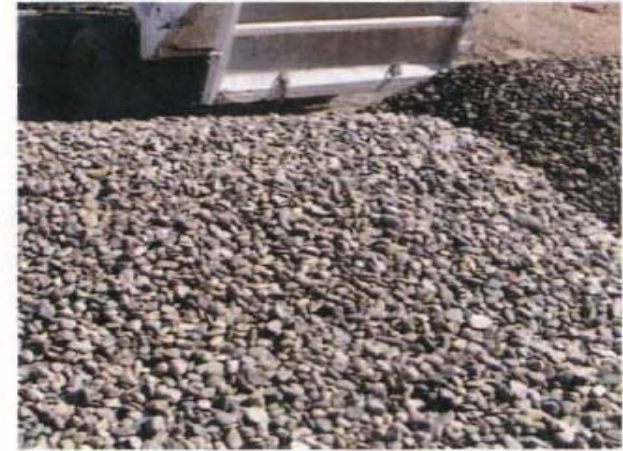
Gravel – coarse aggregate
