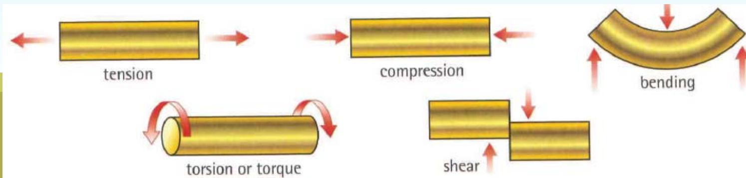
Bending comprises two opposite stresses: tension and compression. This is shown in the diagram of a **simply supported beam**. As a result of the bending force, the lower half of the beam is **in tension** and the upper half is in **compression**. These opposite stresses reach their maximum at the upper and lower surfaces of the beam, and progressively decrease to zero at the **neutral axis** - an imaginary line along the centre of the beam which is free from stress.
