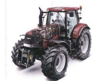
The Case-IH Puma CVX tractor is equipped with continuously variable transmission.
