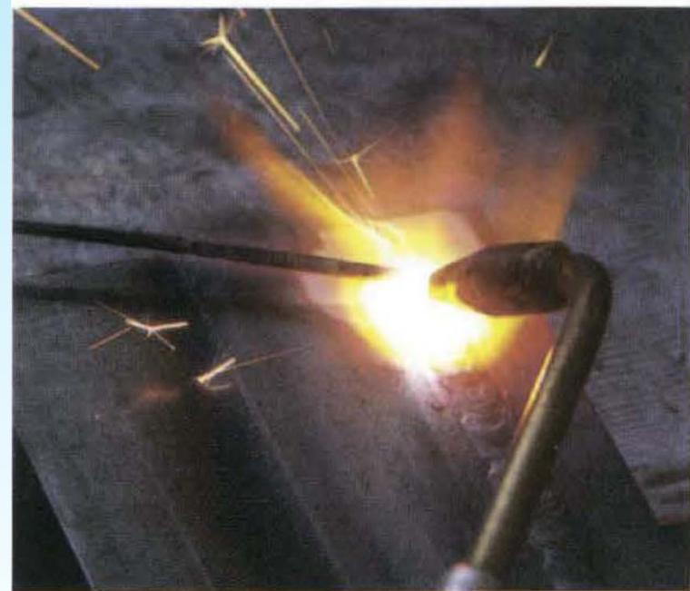
Gas welding using oxyacetylene
